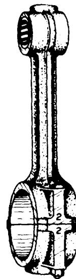
Figure 11B-139. Connecting Rod Markings
